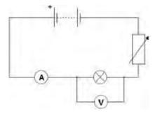
battery in series with bulb and ammeter
